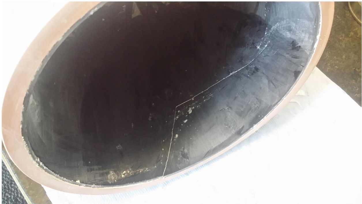
Figure 15: Cracked Stycast after cold-cycling of initial copper bonded absorber
