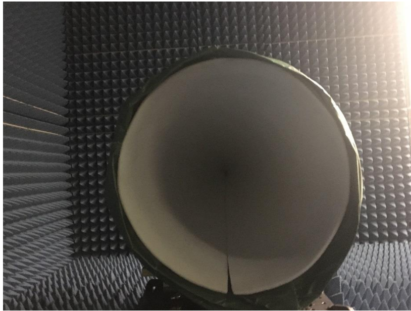
Figure 75: Photograph looking into polyethylene insulated blackbody. The seam in the polyethylene can be seen towards the bottom of the cone.
